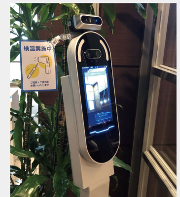
Installation of thermographic monitors to measure temperature (Fukuoka Realty office entrances)
